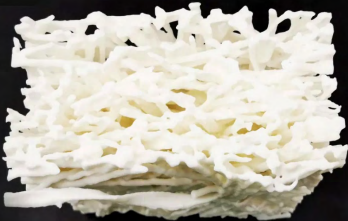
Figure 2: Filtration media structure produced by Farsoon 403P. Image courtesy: MANN+HUMMEL
