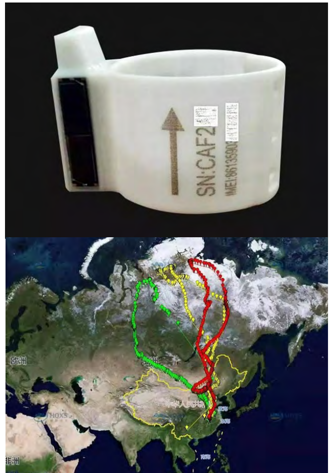
Figure 3: (Top) The 3D printed trackers for swans produced by Farsoon's plastic laser sintering technology, designed by Hunan Global Messenger. (Bottom) The tracked migration routes of three Tundra swans (Image courtesy: Nanji Wetland Conservation Association)
