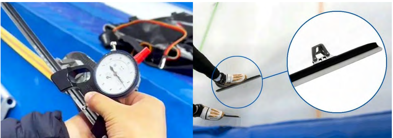
Figure 2: The speed skating technician measures the radius of Farsoon's 3D printed blades. Image Courtesy: Farsoon Technologies
