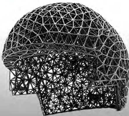
Figure 2: 3D printed bobsled helmet lining produced by Farsoon's Flight® Technology (left) & the helmet used in racing (right). Image Courtesy: Farsoon Technologies
