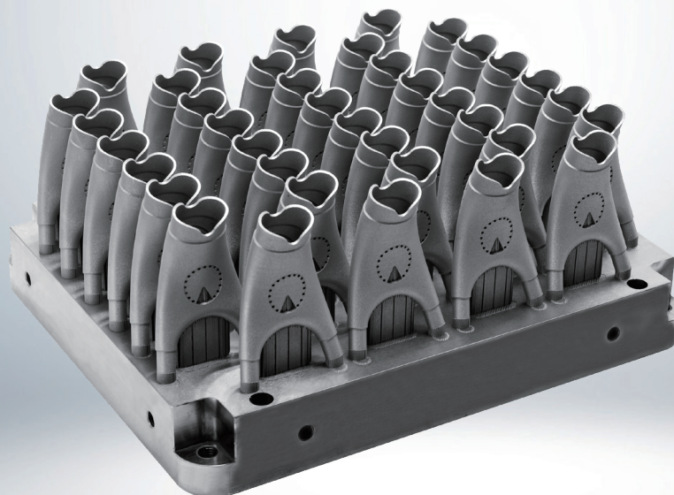
BIKE YOKE MATERIAL: Ti6Al4V SYSTEM: FS350M-4 PRINT TIME: 24H
